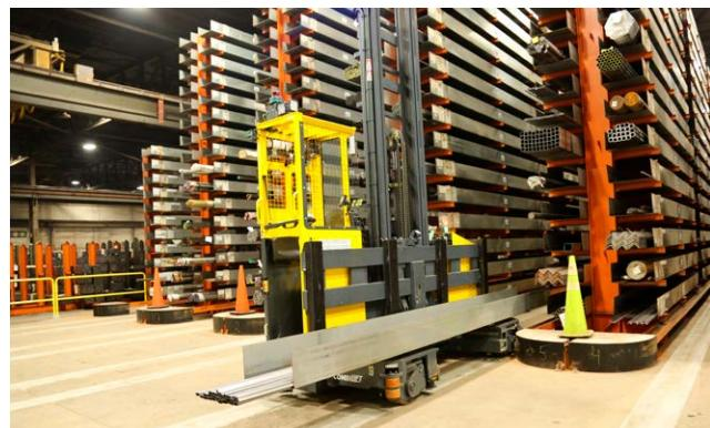
The first autonomously guided side-loader with optional manual override operation. Safely and reliably deliver long loads in narrow aisles around the clock with the new Combi-AGT. Perfect for operation in cantilever racking.
